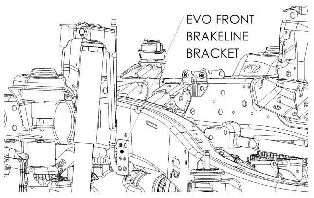
18. Install factory brake line to the new lower location on the EVO brake line extension bracket. Be very careful moving line into new location. The factory hardline will need to be slightly manipulated to be relocated. Do not use tools or pinch/crack the line.
