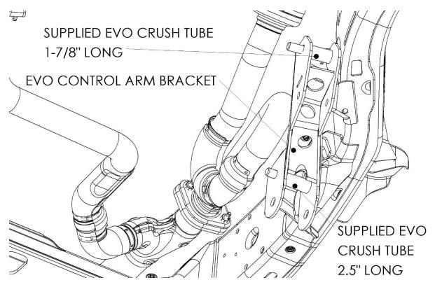
Rotate control arms back into their new location on the EVO Control arm relocation brackets. Use Supplied M12 bolt, washers and nut for upper control arm mount and 5/8 bolt, washers, nut for lower control arm mount.
