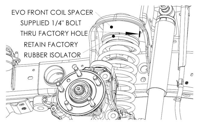
16. Reinstall factory coil spring and rubber isolator on top of coil into its original location on both the frame and axle. Isolator will now be seated on the EVO coil spacer. Axle may need to be lowered to install.
