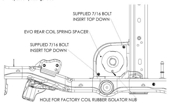
38. Reinstall driver and passenger side coil springs into place keeping factory rubber isolator on top of spring. Be sure to align nub on isolator so that it inserts into hole in EVO brackets. The spring isolator will now be resting on the EVO coil spring spacer.
