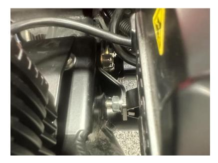
1. Remove the 7/16" nuts and washers using a 5/8" socket and wrench and install the lower fog light bracket that kicks towards the center of the vehicle.
