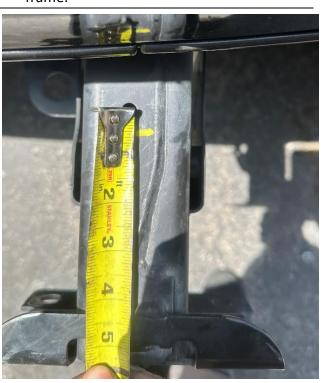
JK ONLY: The first cut line should be drawn 1.5" from the center of the top hole. The second cut line should be on each of the front body mounts, 2" down from the top of the frame.
