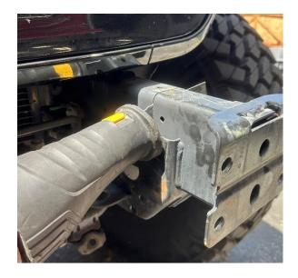
8. Remove all brackets apart of the front frame horns as well as the sway bar mounting brackets.
