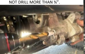
25. Using the same bolt removed earlier install through the factory rubber isolator and into the newly drilled hole. Tighten all sway bar bolts.
