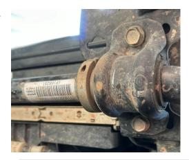
6. JL/JT ONLY: Mark cut lines as shown. The first cut line should be drawn ½" from the center of the top hole. The second cut line should be on each of the front body mounts, 2" down from the top of the frame.
