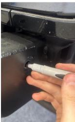
14. Remove the bumper and drill the 8 side holes that were marked in the previous step with a ½" drill on the outside of the frame and a ¾" drill bit on the inside of the frame.
