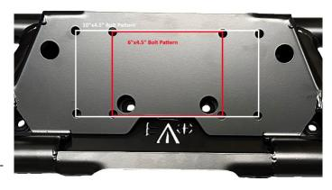
18. After installing the winch (if applicable), install the six 5/16" flat head cap screws to mount the skid plate to the bumper.
