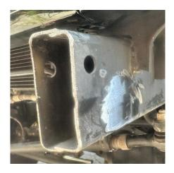
10. JL/JT ONLY: Grind / sand down the sway bar bushings so they are flat with the brackets
