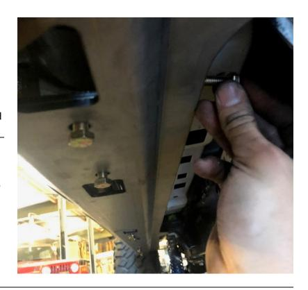
When all bolts in parts are installed, apply an inward pressure on bomber, tighten body mount bolts.
