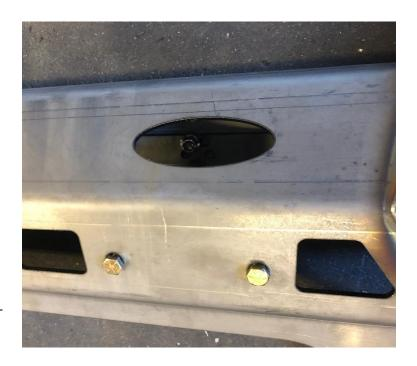
12. Install rear body mount plate to bomber using 3/8" hardware.
