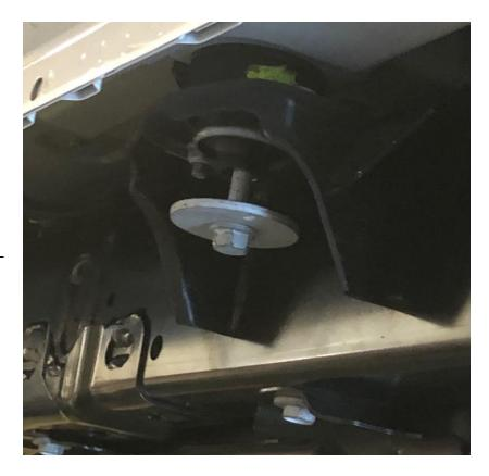
10. Loosely preassemble inner seam mounts to main bomber rails. The inner seam mounts with the 4-center hole pattern will be used at both front and front/middle locations. The inner seam mount with the 2-center hole pattern will be used at the rear and rear/middle locations.
