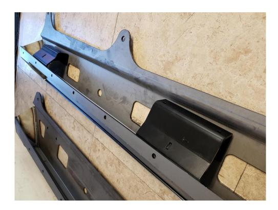
4. Using the supplied 3/8" hex head hardware, loosely install all 6 bolts from bottom up at all 3 inner seam mount locations (2 bolts each mount). It is best to tighten these to the point just before getting tight, loose but almost tight. This will save time later when tightening to vehicle.
