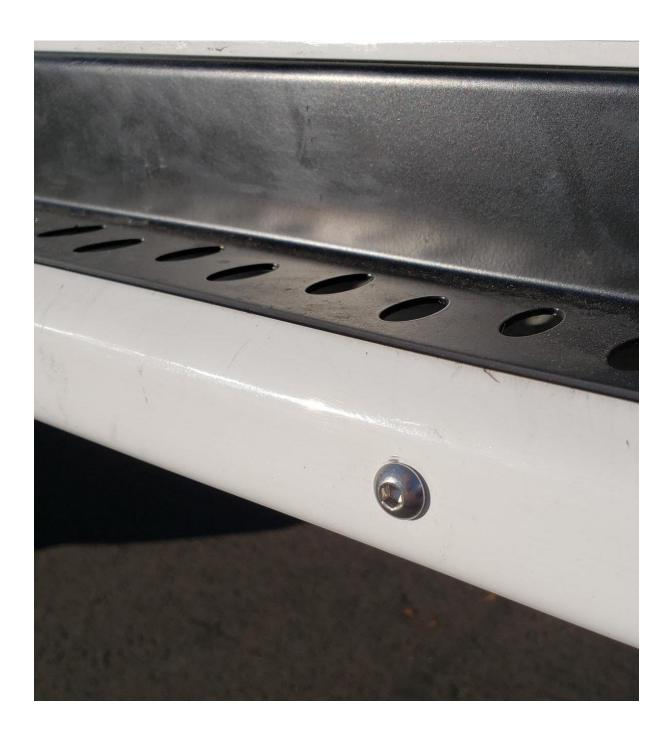
3. Loosely preassemble the inner seam mount brackets to main rocker rails. The inner seam mount brackets with the **4-bolthole pattern on top will be used at both the front and middle locations** on each side rail. The inner seam mount with the **2-bolthole pattern on top will be used at the rear location only**.
