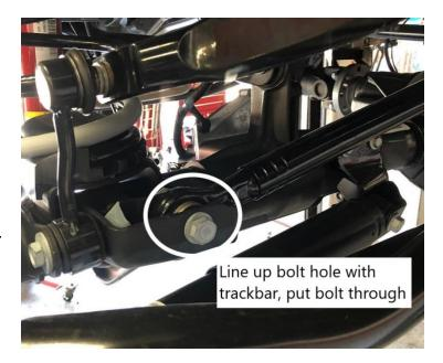
While on ground under Jeeps own weight at ride height, torque all control arm bolts, uppers, lowers at frame and axle. Torque all shock bolts at frame and axle. Torque front trackbar bolt. Check and torque all other bolts. Use chart below for supplied hardware. Use factory specifications for factory hardware.
