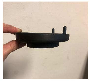
Note: Make sure factory coil seats stay in the factory locations, Left coil seat on the left and right on the right, etc. Also make sure that the rubber pins insert into holes on coil brackets.
