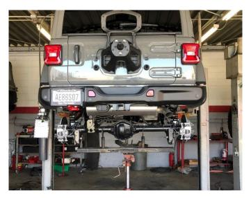
4. Remove both driver and passenger side swaybar links bolts at axle and swaybar removing swaybar links and rotate sway up and out of the way.
