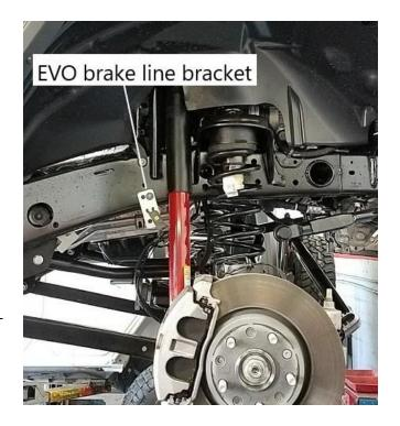
13. Reinstall shock at axle per factory specifications. If you are installing shock extensions. Do so at this time. Follow instructions for that kit. If you are installing new shocks, follow shock manufacturers specifications and install shocks at both upper and lower mounting locations. Torque to factory specifications.
