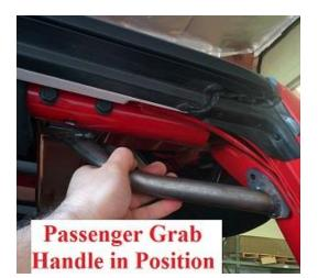
2. Keeping the grab handle positioned, mark the holes to be drilled.
