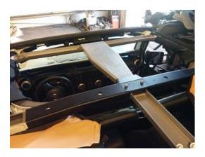
8. Fit the EVO MFG B-Pillar Plates on the corners with the factory plates over them, as shown. If equipped, plug the GPS unit back into the wiring harness.
