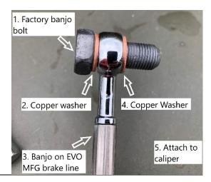
42. Using a socket, secure your new stainless steel break line to the break caliper using factory hardware, tighten the banjo bolt to 276 in. lbs. of torque (at caliper hard line elbow extends towards rear of vehicle and angled up as much as possible.)
