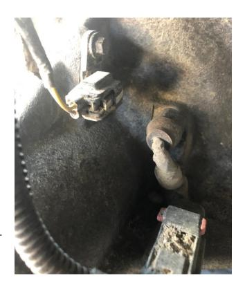
Support axle with jacks and remove rear sway bar end links from vehicle. (upper stud end on sway bar link has hex key on end of the stud to prevent rotation while removing nut).
