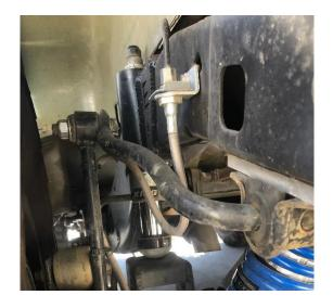
41. Install new copper crush washers on to the factory banjo bolt, Insert the factory banjo bolt with copper crush washer on through the banjo of the new stainless-steel brake line, then slip another copper crush washer on.
