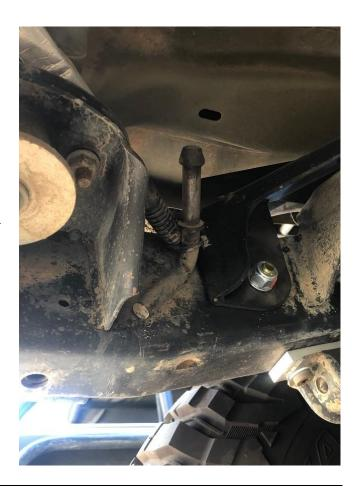
13. Using a jack, carefully apply pressure to rear tub lifting rear of body from frame. There needs to be about a ½" gap between body and frame.
