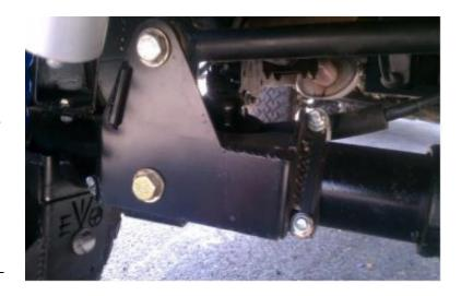
29. Install bumpstop extension to axle. Angle of pad should be faced to forward of axle. Use supplied 5/16" hardware.
