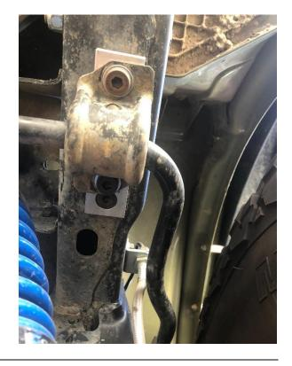
38. Assemble rear swaybar endlinks. Apply WD40 into endlink tube. Tap hourglass into endlink ends with mallet. Insert sleeve into center of hourglasses.
