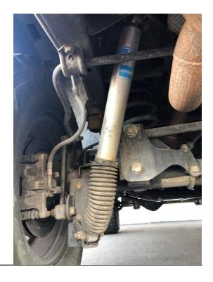
7. Lower axle until springs can be removed. Remove rear springs and upper/lower coil isolators.
