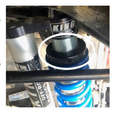
Once vehicle is on the ground, if you have the EVO MFG upper control arms then adjust them out until pinion is facing the transfer case. The angle of your driveshaft and angle of your pinion should have zero degrees difference between the two. The driveshaft face and pinion face should be parallel with each other.
