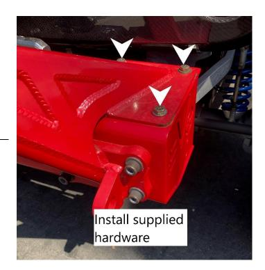
4. Using supplied hardware attach Stinger to the top of the Bumper.
