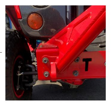
3. Using the upper holes as a reference, drill through the holes, into the top of the bumper.
