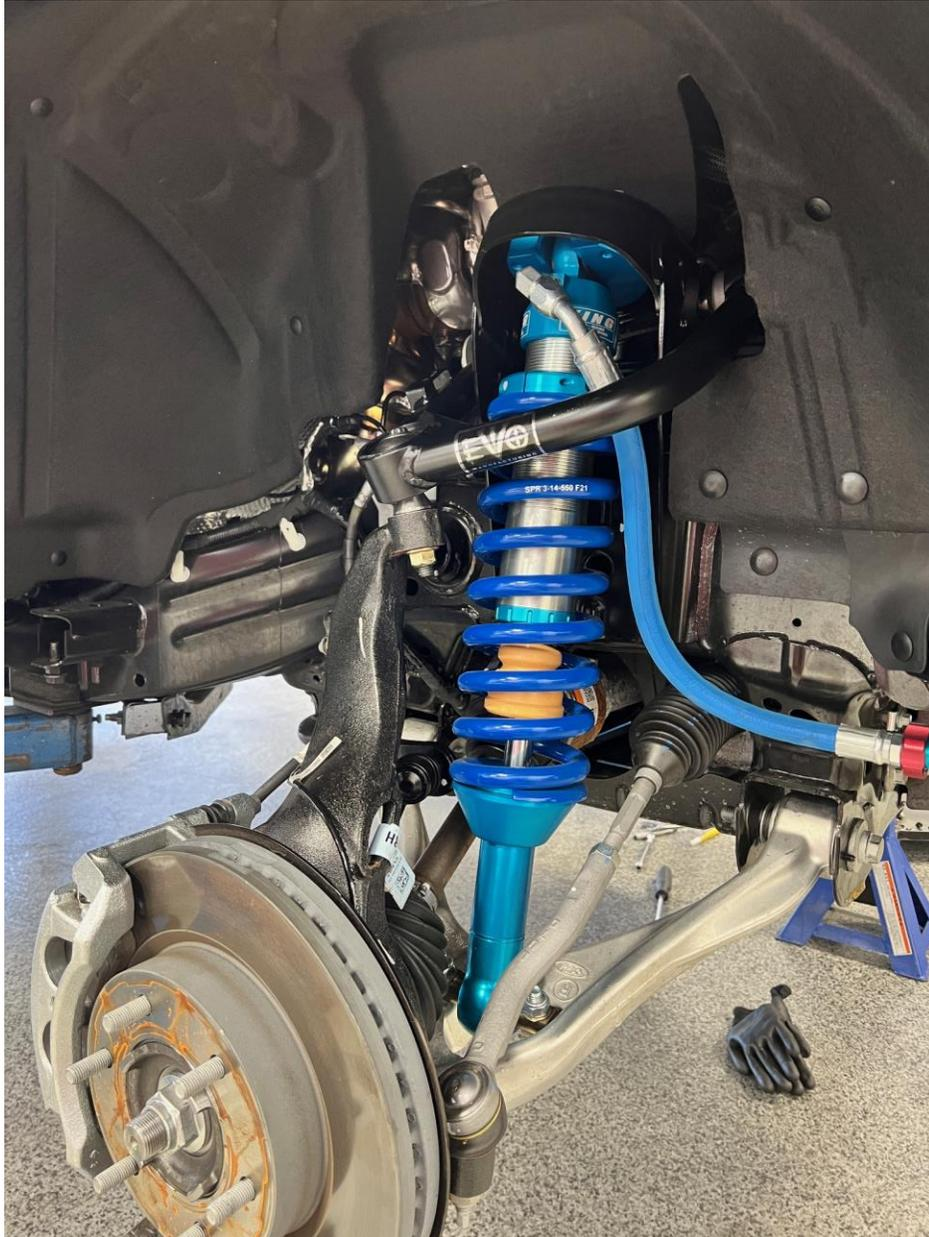
7. Install O-Ring onto Billet Bearing cap and install to EVO Control Arm. Small spray of lubricant like WD40 can help installed into arm groove.
