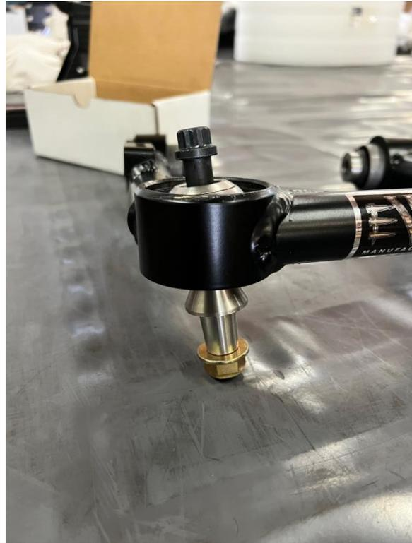
4. Install EVO Front Upper Arm Assemble to frame in factory location using factory bolt. (note cap on control arm bearing/spindle end should not be installed at this time).
