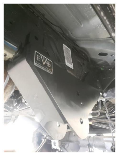
6. Using a ½" and ¾" Drill. Drill Smaller Inside frame holes with ½" and drill larger outside frame hole side with ¾". Depending on equipment, may require you to remove brackets and drill at marked locations.
