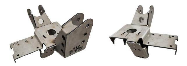
This instruction is to be used as a general guide of assembly on various axles. Use original axle measurements for placement of bracketry, adjust for personal application. Radius openings on bracketry are 3.5" diameter, grinding can be done to adapt to others.
