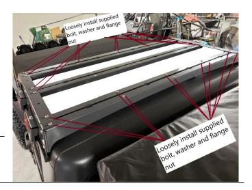
6. Using supplied 5/16" bolt, washer, flange nut. Install upper bolt plate and lower bolt plate as shown. Install upper bolt plate from inside of main plate through slot toward the outside. Tighten bolts. Do this at all 4 ends.
