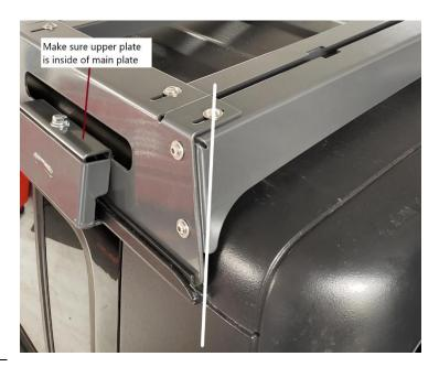
11. Insert bolt and washer from top down of upper mounting plate and thread into outer rail mount. Lower edge with trim should be grabbing underside of hardtop drip rail.
