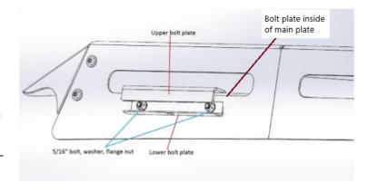
Using your nutsert installation tool and tool specific installation guide, install nutserts onto the outer rail mounting plate. Use picture as reference.
