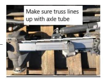
5. Ensure truss sections seat in place and adjust as needed. Some taps with a mallet may be necessary to align.
