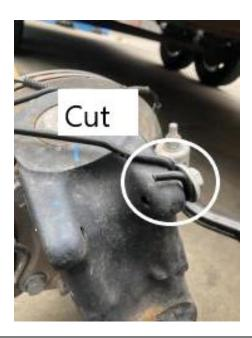
3. Remove bolt holding metal brake line retaining wire and push out of the way.
