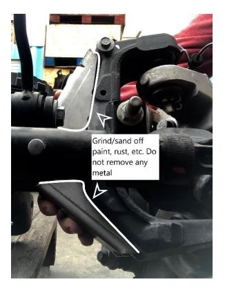
5. Place Upper Gussets in place on both driver and passenger side. Make sure that C2's seat fully against spring perch. Tap with rubber mallet if required. Some grinding of bracket may be necessary to fit on axle.
