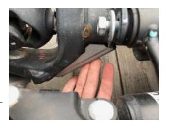
7. Weld gussets in no more than 1 inch increments alternating from driver to passenger sides after every incremental weld. After welding one increment, let welded surface cool before alternating to the opposite side.
