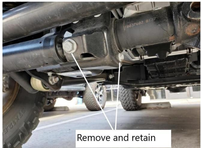
4. Remove upper factory FAD skid bolt directly above right side control arm bracket. Retain.
