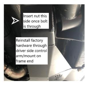
• All bolts need to be tightened after procedure, make sure to tighten bolts after putting vehicle safely on ground, chalking tires, and in park, under vehicles own weight at ride height.
