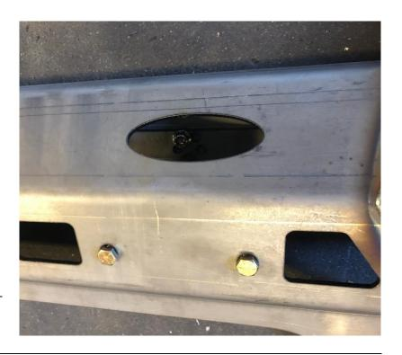
4. Lift bomber rockers onto jeep (with help from another person or jack) and guide factory bolts through bomber and back into factory locations. Do not tighten.
