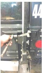
9. EVO MFG recommends drilling a ¼" hole in the foot of your jack as shown in the photo. This hole will allow you to secure your jack with the supplied square neck carriage bolt and wing
